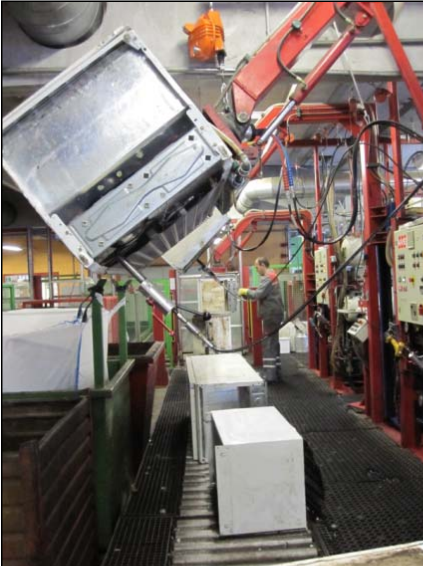
Photo 11 Step 1 of CFC recovery from refrigerators (Source: Öko-Institut 2010)
